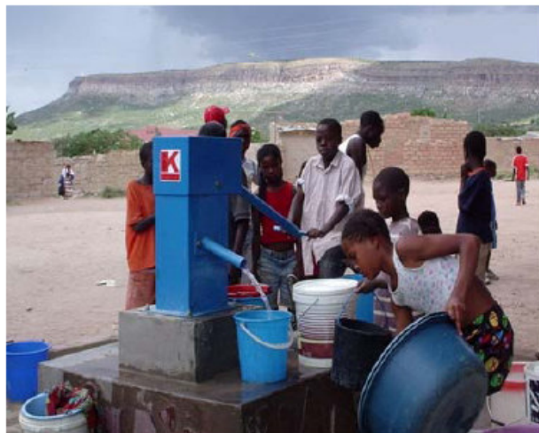
Fig. 2. The Afripump with a locally made blue box in South Angola, on a rehabilitated borehole.
