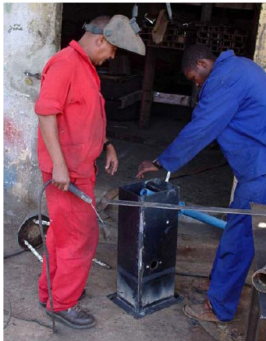
Fig.8 Partial local production is possible; a local metal workshop in Angola welcomes the extra business and can produce many Afripump parts.
