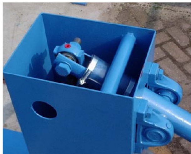
Fig. 4. The heavy duty bearings of the Afripump handle are maintenance free with a 25+ year lifetime.
